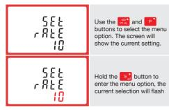
Use the price and pributtons to choose the desired pulse rate. To save the new setting, hold the c button for 3 seconds until the selection stops flashing
