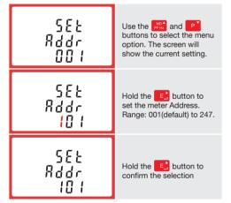
Use the the press the press the terms to choose the necessary number, then press the the button to move along to the next number. To save the new setting, hold the the button for 3 seconds until the selection stops flashing
