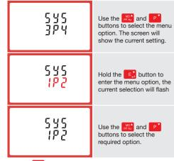
Hold the E button to confirm your adjustment. Hold th button for 3 seconds to exit the set up menu.
