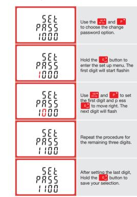
Hold the VA button for 3 seconds to exit the set up menu.
