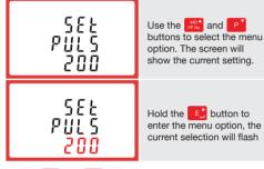
Use the *mathefactory* and *buttons to choose the desired pulse* rate. To save the new setting, hold the **E** button for 3 seconds until the selection stops flashing
